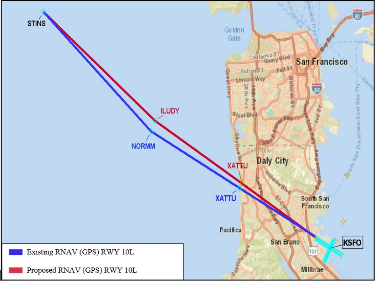
Figure 4. Proposed Amended RNAV (GPS) RWY 10L
