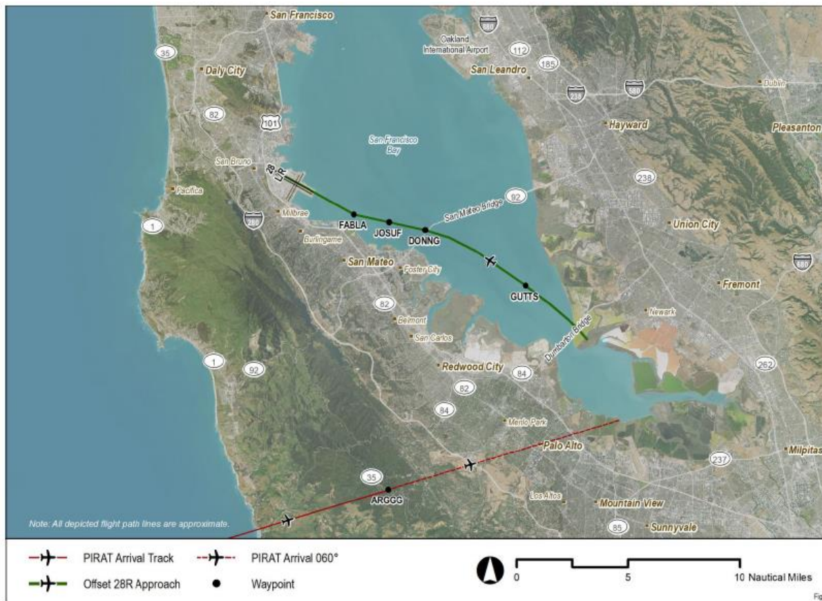
Red line: PIRAT Arrival track and 060° heading. Green Line: suggested offset path to 28R until passing the San Mateo Bridge
