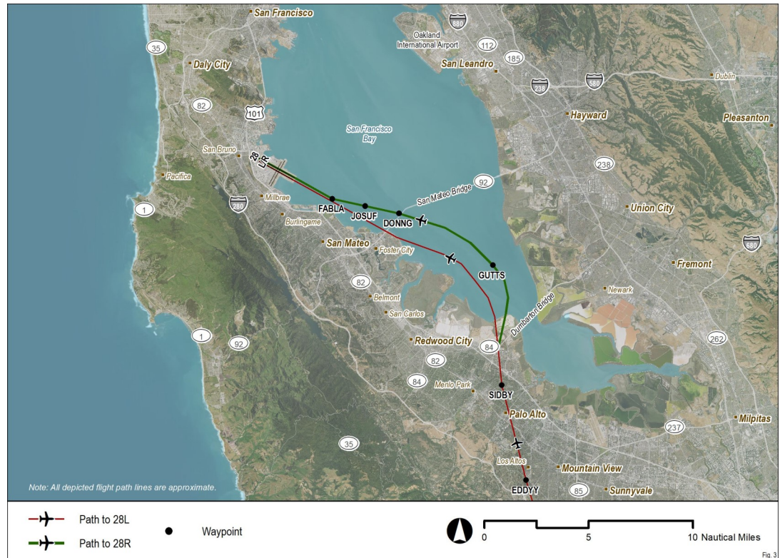
Green line: suggested offset path to 28R until passing the San Mateo Bridge
