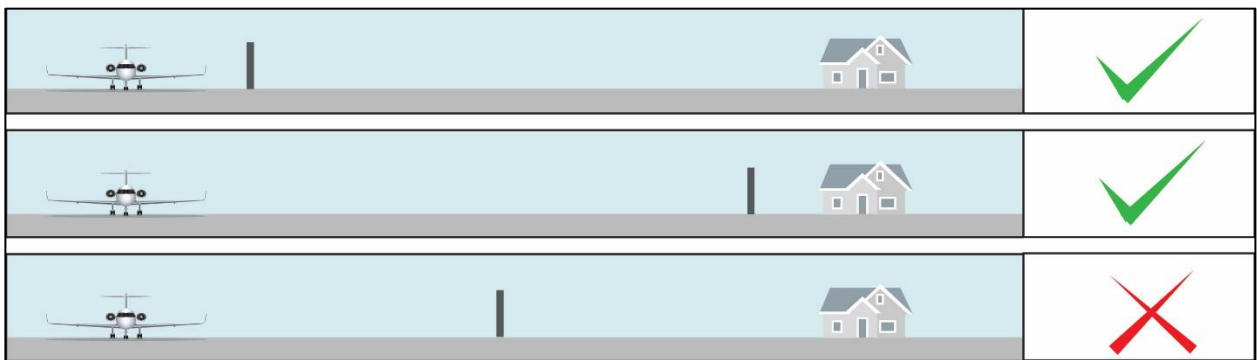
Figure 3. Noise Barrier Placement
