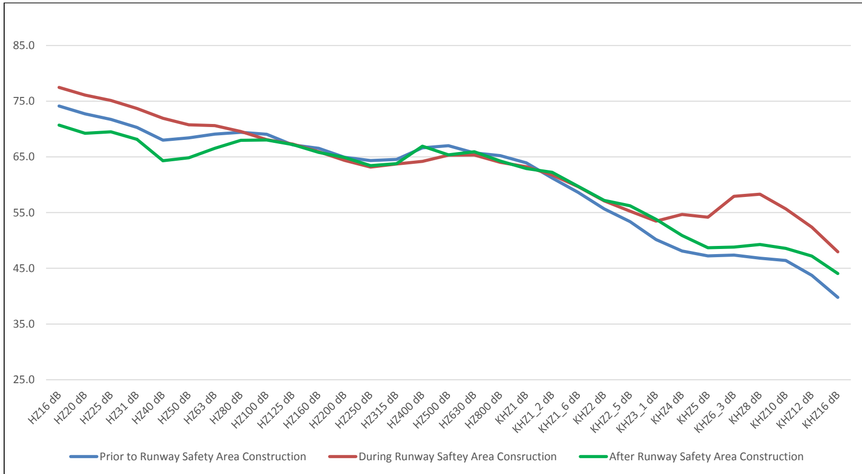
Figure 6. Spectral Noise Analysis Runway 01L - Prior, During and After Runway Safety Area Construction
