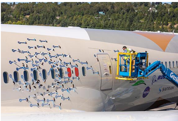
Figure 6. Microphones attached to the 787-10 Dreamliner ecoDemonstrator
