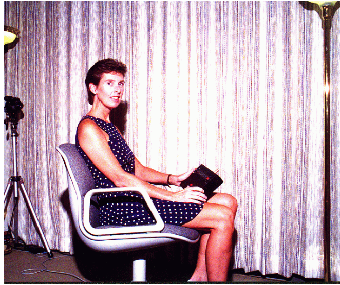
Figure 11 Interior view of low-frequency test facility test subject chamber, showing seated test participant holding response box used to record subjective judgments.
