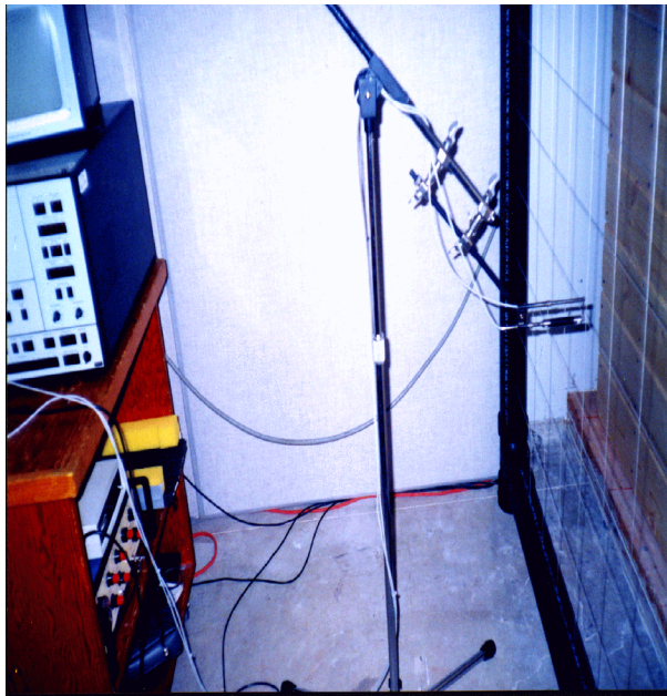
Figure 53 Measurement of sound intensity at one grid point location.
