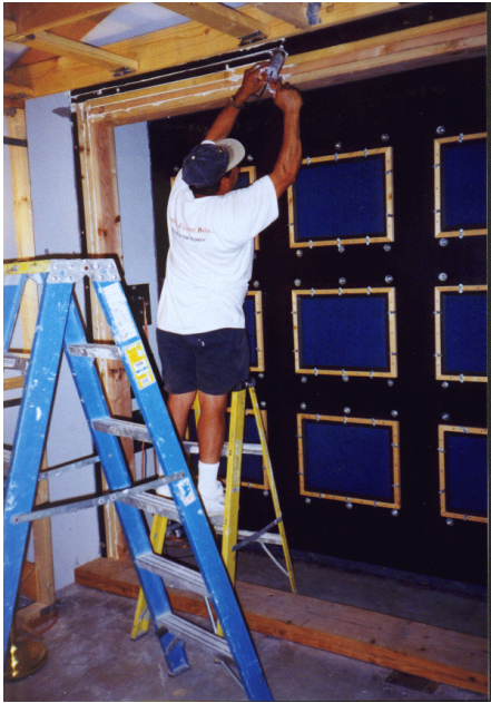
Figure 48 Sealing mounting framework for test articles.
