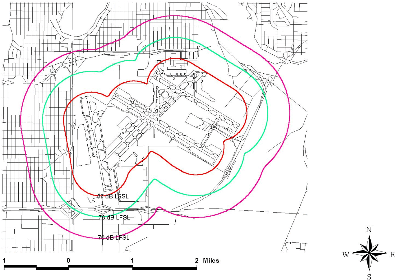
Figure 4 Contours of low-frequency sound levels due to thrust reverser application (per 3 February 2000 revision of Sutherland model).
