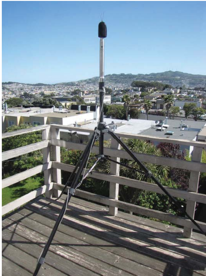
Figure 1 – Microphone and tripod on top floor rear exterior deck.
